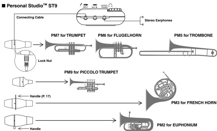
Before connecting the cable and attaching the Pickup Mute™, make sure the power is switched OFF and the earphones are removed from your ears.
