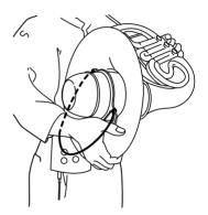
As shown in the illustration, lightly support the handle in the middle of the Pickup Mute™ with the ball of your thumb while holding the instrument at the bell rim with your other fingers. The handle also features a ring for a wrist band, allowing you to hang the Pickup Mute™ from your wrist (just like any other mute) while emptying the horn. (Wrist band is not included.)
