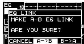
Move the cursor to the button and then press the knob to link the EQ settings.
