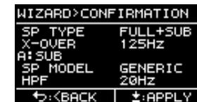
After confirming the setting is appropriate, press the main knob to actually apply the set value.
