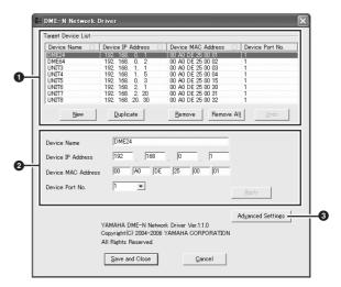
In order to use the YAMAHA DME-N Network Driver, all computer network devices (hubs, routers, etc.) must be properly connected and configured. Use a cross cable if you will be directly connecting a DME64N/24N to the computer without using any other network devices.
