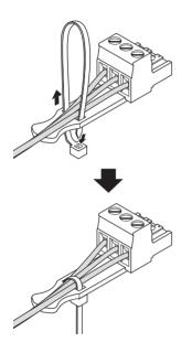
5 Insert the Euroblock plug into the AES/EBU [IN] or [OUT] connector of the MY4-AEC.
