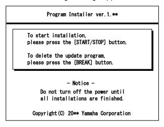
4) When the following message appears, press the [START/STOP] button to start firmware installation. A progress bar for installation will appear.
