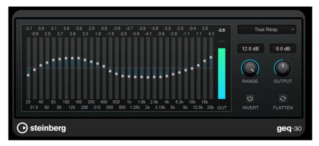
Each band can be attenuated or boosted by up to 12 dB, allowing for fine control of the frequency response. In addition, there are several preset modes available that can add color to the sound of GEQ-30.
