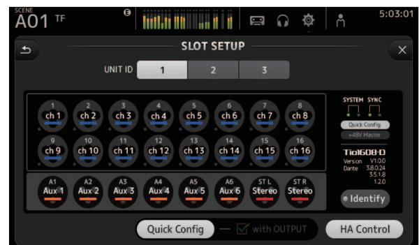
7. To assign the Tio1608-D inputs to the TF series mixing console, set the input select on the console's INPUT screen to "SLOT".
