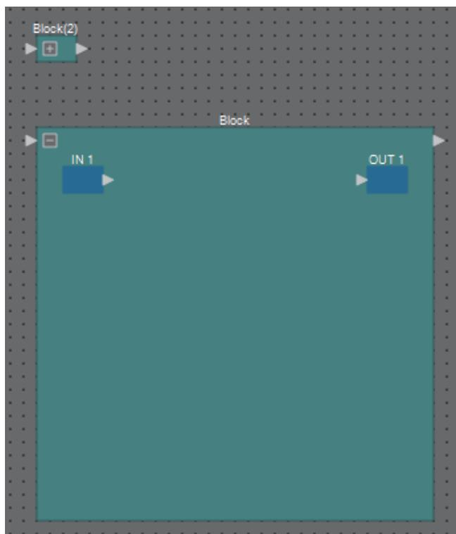
Components in a block can be placed, connected, and edited in the same way as in a design sheet. With a block selected, you can drag and drop the top, bottom, left, or right corners to expand or shrink the block. With an expanded block selected, you can drag and drop the top, bottom, left, or right edges to move the block on the design sheet.
