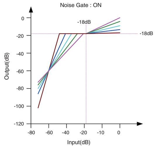
If the input is below the Threshold value, the output is adjusted so that the output is  $-18$  dB when it reaches the Threshold value.
