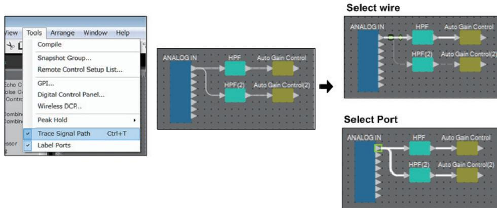
If the signal path is connected but no audio signal flows because it is turned OFF or the level is minimized, the signal path is shown as a dashed line.
