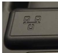
Connect the other end of the Ethernet cable into a jack providing PoE or a PoE adapter.
